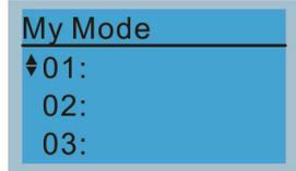
Click F4 in parameter setting page, the parameter will save to My Mode. To delete or correct the parameter, enter this parameter and click the "DEL" on the bottom right corner.
