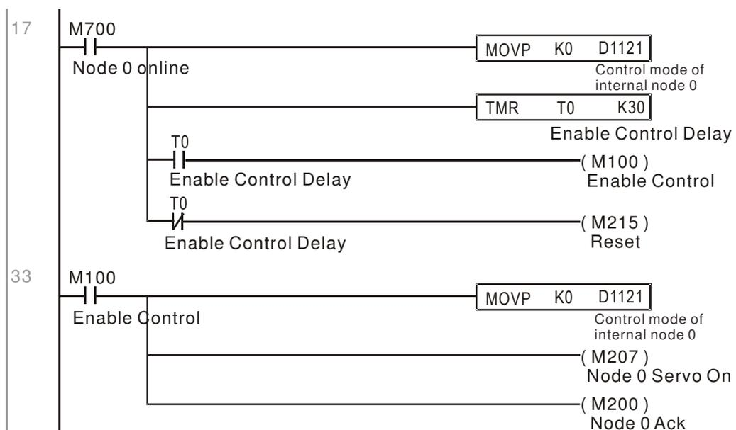
It is required slave station 1 maintain forward rotation at 30.00Hz for 1 sec., and maintain reverse rotation at 60.00 Hz for 1 sec., and repeat this cycle continuously.
