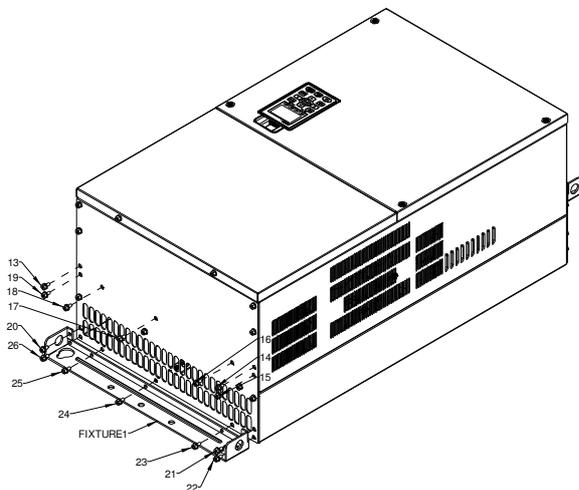
4. Install Fixture 1 by fasten screw 13 ~26
