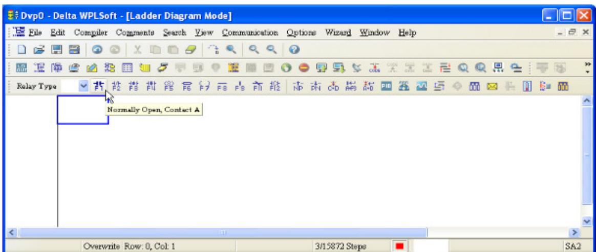
3. After the name of the input device and the comment dialog box have appeared, the device name (such as "M"), device number (such as "10"), and input comments (such as "auxiliary contact") can be selected; press the Confirm button when finished.
