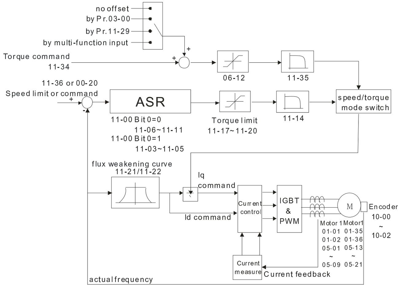
TQC Sensorless control diagram is shown in the following diagram:
