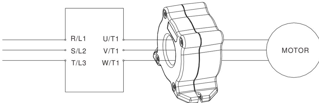
**Note 1:** The table above gives approximate wire size for the zero phase reactors but the selection is ultimately governed by the type and diameter of cable fitted i.e. the cable must fit through the center hole of zero phase reactors.
