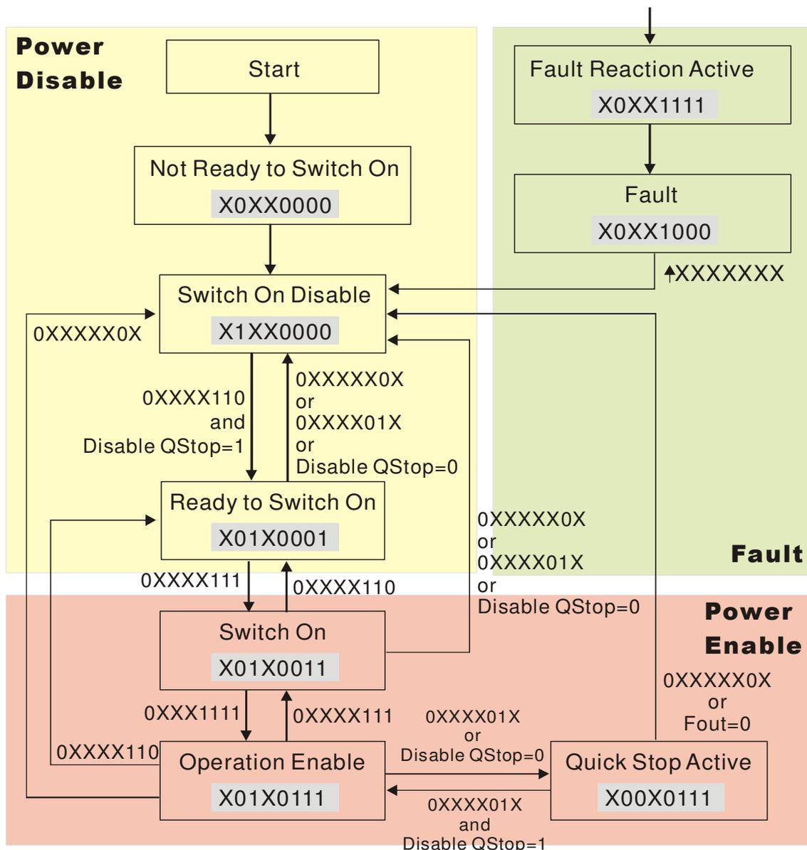
Set command 6040 =0xE, then set another command 6040 =0xF. Then the motor drive can be switched to Operation Enable. The Index 605A decides the dashed line of Operation Enable when
