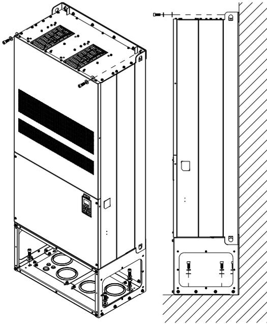
Secure the drive from the internal.
