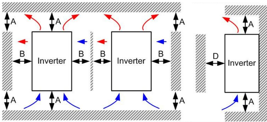
Multiple drives side-by-side vertical installation (Frame A~H)
