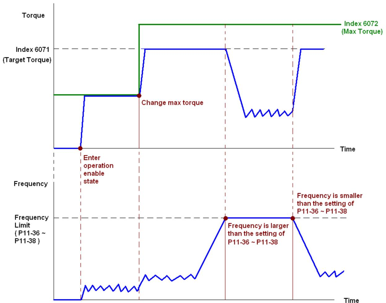
NOTE: The standard DS402 doesn't regulate the highest speed limit. Therefore if the motor drive defines the control mode of DS402, the highest speed will go with the setting of Pr11-36 to Pr11-38.
