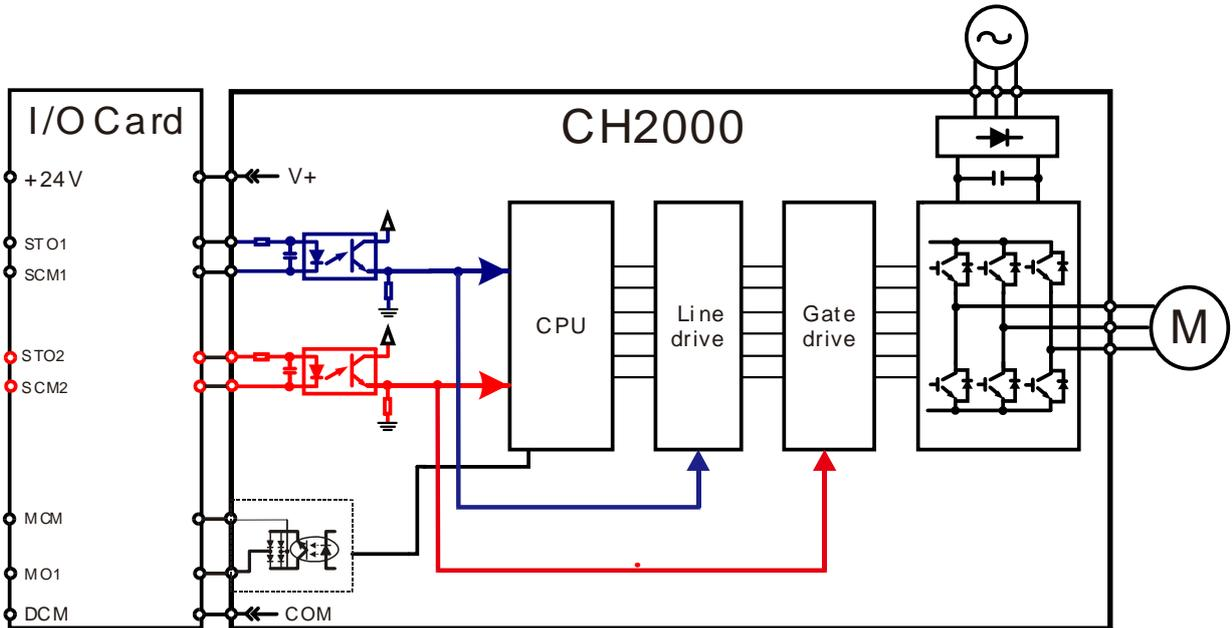
17-3-2 In the figure below, the factory setting for +24V-STO1-STO2 and SCM1-SCM2-DCM is short circuit:
