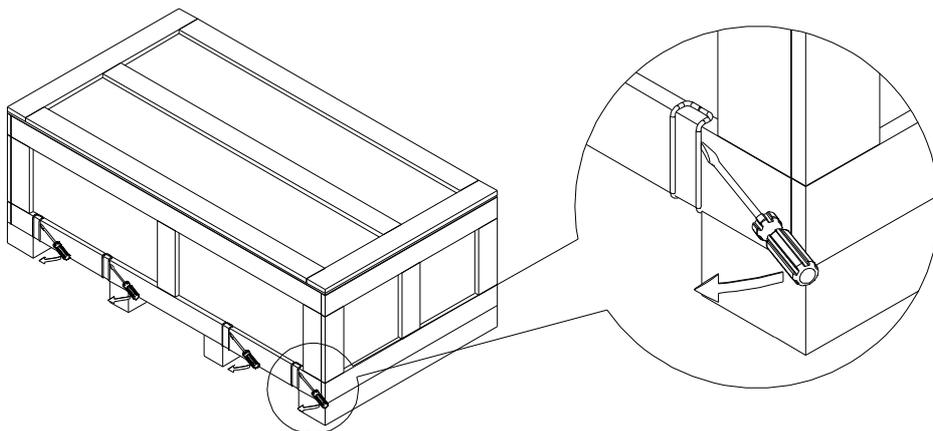
Remove the crate cover, EPEs, rubber and manual.
