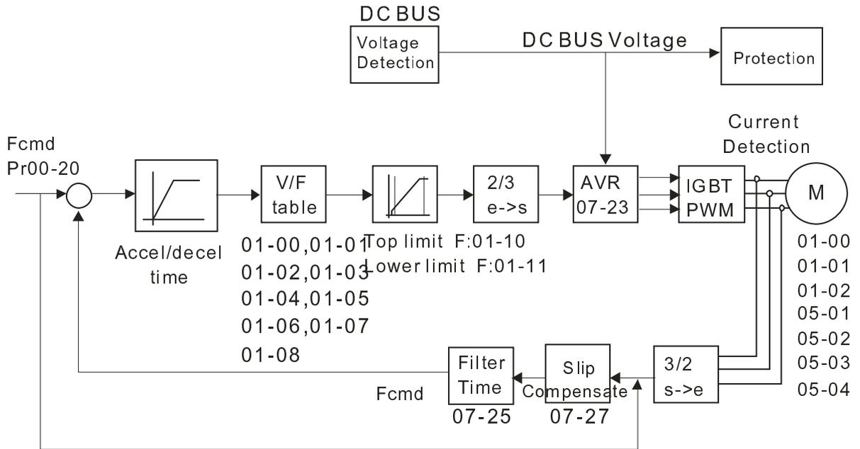
When setting Pr.00-11 to 3, the FOC PG control diagram is shown as follows.
