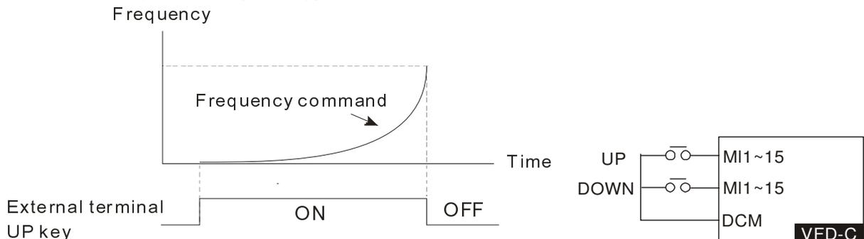
Pr.02-09 set to 1: it will increase/decrease frequency command (F) by the setting of acceleration/deceleration (Pr.01-12~01-19) and only be valid during operation.
