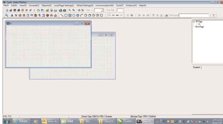
2. Numeric/ASCII Display : To add a Numeric/ASCII Display object to a screen, double click on the object to set up Related Devices, Frame Setting , Fonts and Alignment.
