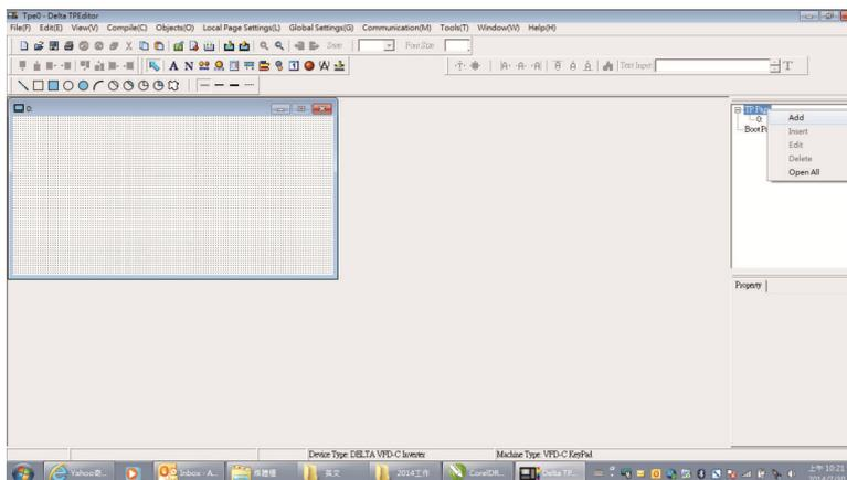
2. On the bottom right-hand corner of the HMI, click on a page number to edit or go to VIEW >HMI page to start editing main page. As shown in the image, the following objects are available. From left to right: Static Text, ASCII Display, Static Bitmap, Scale, Bar Graph, Button, Clock Display, Multi-state bit map, Units, Numeric Input and 11 geometric bitmaps and lines of different width. The application of Static Text, Static Bitmap, and geometric bitmap is the same as the editing startup page.
