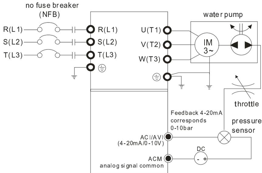
1. Pr.00-04 is set to 10 (Display PID analog feedback signal value (b) (%))
