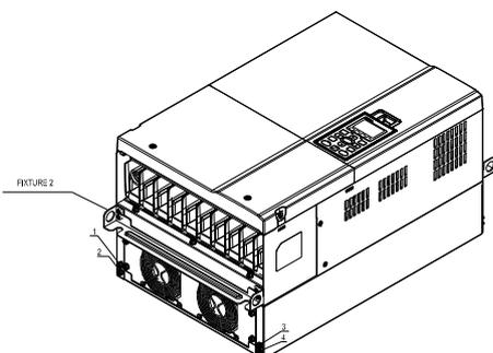
6. Fasten 5 screws (as shown in the following figure). Screw torque: 24~26kg-cm (20.8~22.6lb-in).
