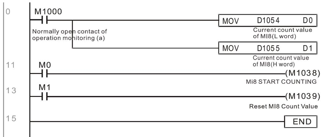
※ When the PLC program defines MI8 for use as a high-speed counter, and also for use in PLC procedures, it must be written to M1038 or M1039, and the original MI8 functions will be disabled.
