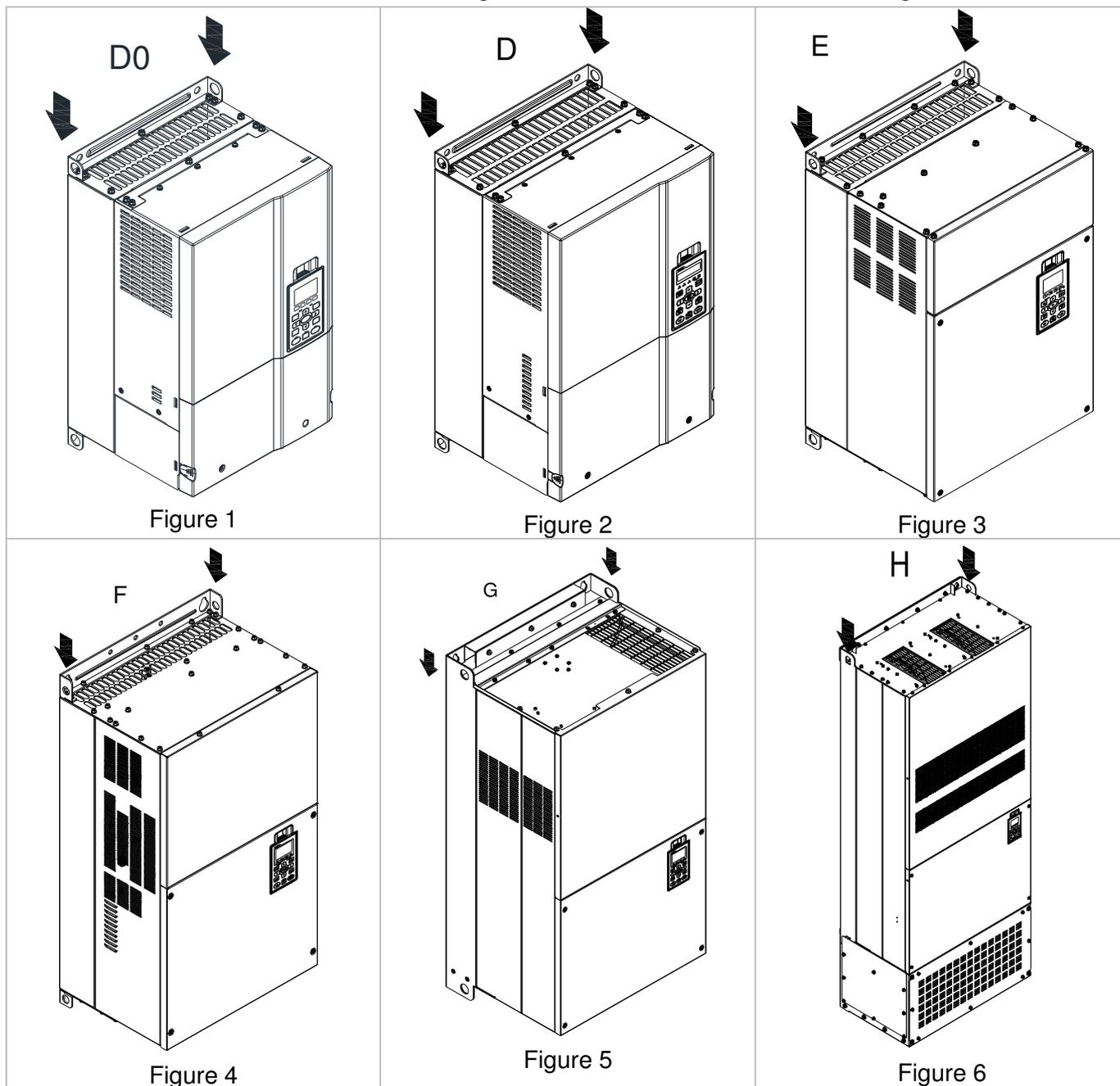
Ensure the lifting hook properly goes through the lifting hole, as shown in the following diagram. (Applicable to Frame D0~E)
