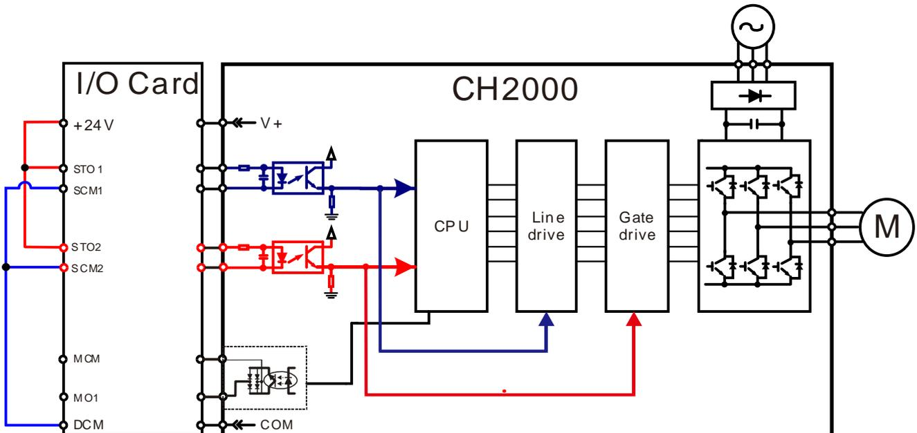
17-3-3 The control loop wiring diagram:
