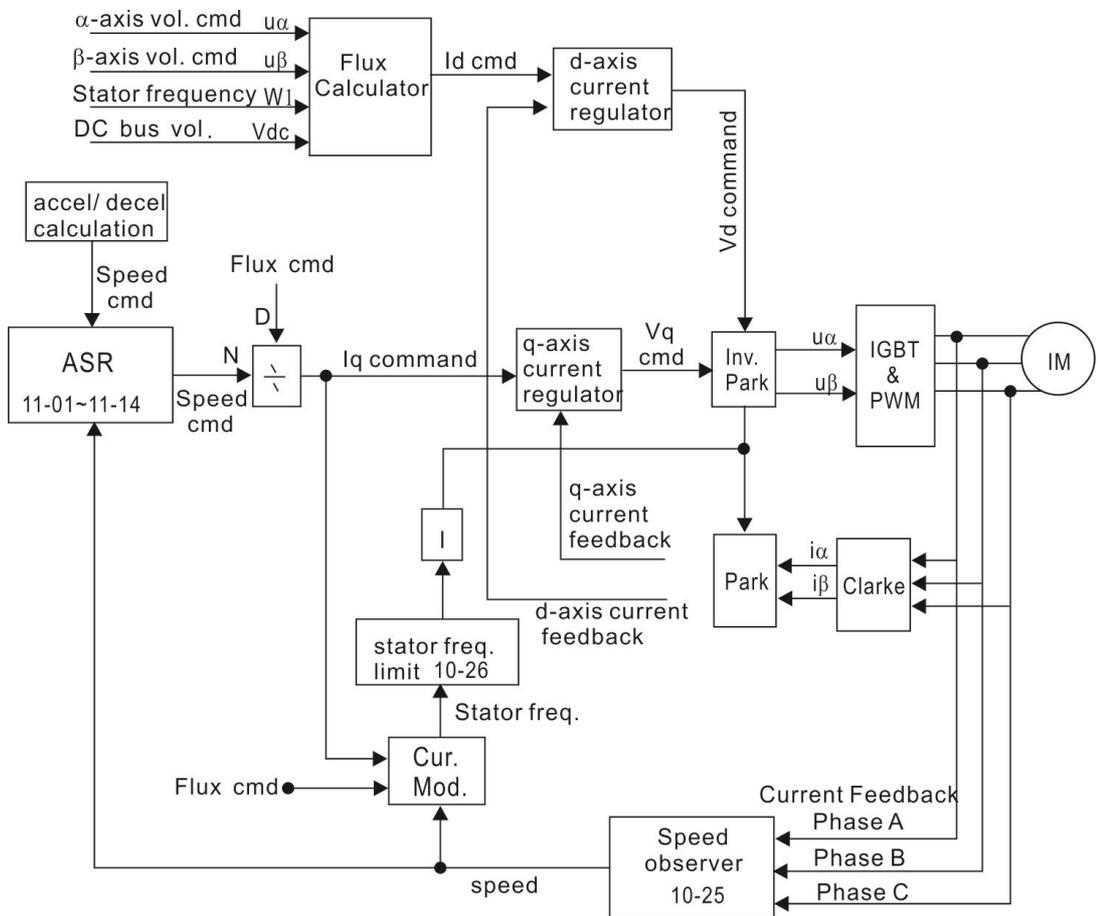
When setting Pr.00-11 to 6, PM FOC sensorless control diagram is shown as follows:
