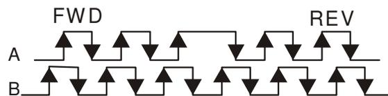
3: Phase A is a pulse input and phase B is a direction input. (L=reverse direction, H=forward direction)
