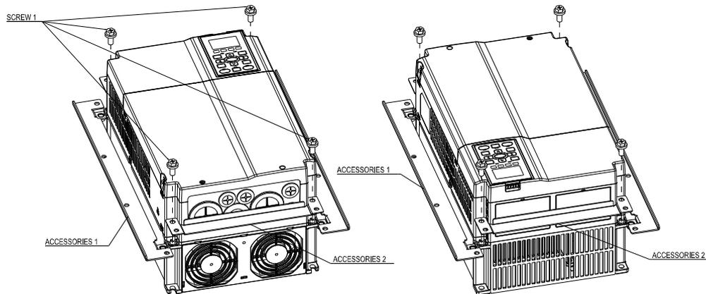
2. Plate installation, place 8 of the screw 2 (M6) through Accessory 1&2 and the plate then fasten the screws. Screw torque: 25~30kg-cm (21.7~26lb-in). (As shown in the following figure)
