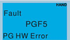
Fault<br>PGF5<br>PG HW Error     | Hardware error of PG Card<br>Check if PG Card is insert to the right slot and parameter settings for encoder are accurate.                                                                                                                                                    |                                                                                                                                                                                         |
