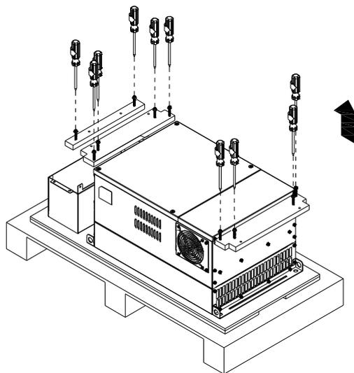
Lift the drive by hooking the lifting hole. It is now ready for installation.
