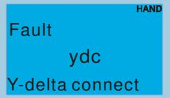
Fault<br>ydc<br>Y-delta connect   | Y-connection/ $\Delta$ -connection switch error                                                                                                                                                                                                                               | <ol style="list-style-type: none"> <li>1. Check the wiring of the Y-connection/<math>\Delta</math>-connection</li> <li>2. Check the parameters settings</li> </ol>                      |
