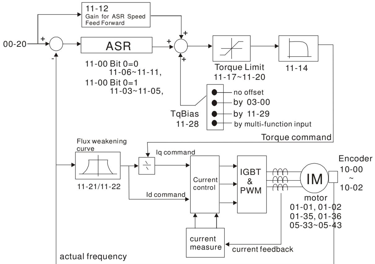
When setting Pr.00-11 to 5, FOC sensorless control diagram is shown as follows.
