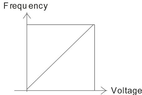
$$F_{command} = [(ay - bias) * gain] * \frac{F_{max}(01-00)}{10V \text{ or } 16mA}$$
