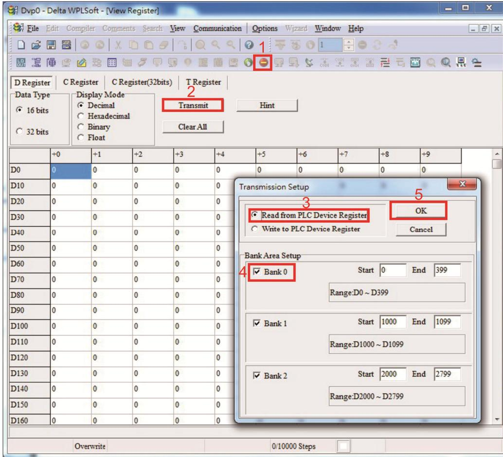
After reading the data, it is necessary to perform some special D settings. Before proceeding, we will first introduce the special D implications and setting range. The CANopen Master's special D range is currently D1070 to D1099 and D2000 to D2799; this range is divided into 3 blocks:
