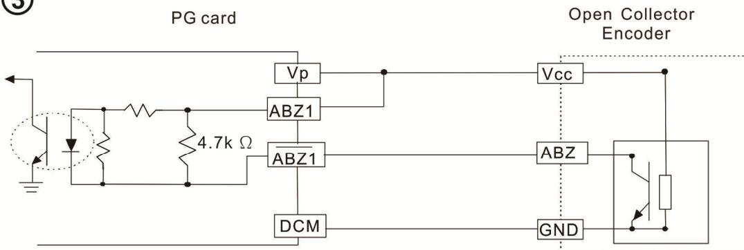
When wiring in this way, if there is a signal on EMC-PG010's A1, B1 and Z1, LED lights is OFF.
