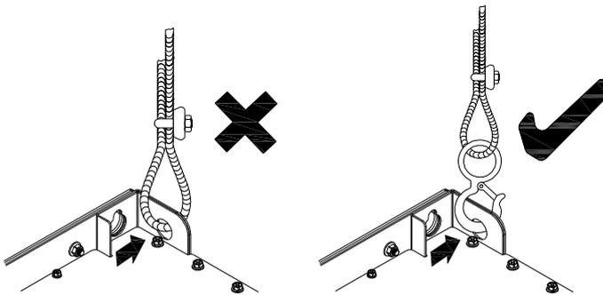
Ensure the angle between the lifting holes and the lifting device is within the specification, as shown in the following figure. (Applicable to Frame D0~E)
