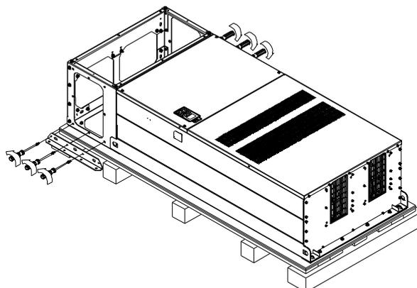
**Secure the drive from the external.** (Skip to the next step if this situation does not apply to you.)
