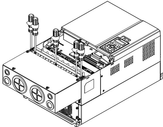
4. Fasten the 2 screws shown in the following figure. Screw torque: 12~15kg-cm (10.4~13 lb-in)
