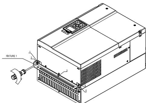
5. Fasten 4 screws (as shown in the following figure). Screw torque: 24~26kg-cm (20.8~22.6lb-in).
