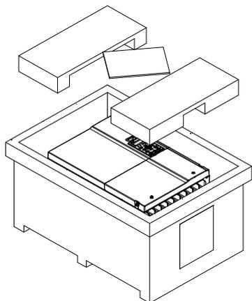
Remove the crate cover, EPEs, rubber and manual.
