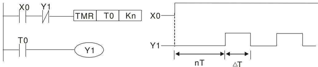
**Example 8: Flashing circuit**
