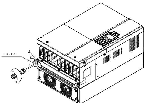
4. Fasten 5 screws (as shown in the following figure). Screw torque: 30~32kg-cm (26.0~27.8lb-in).
