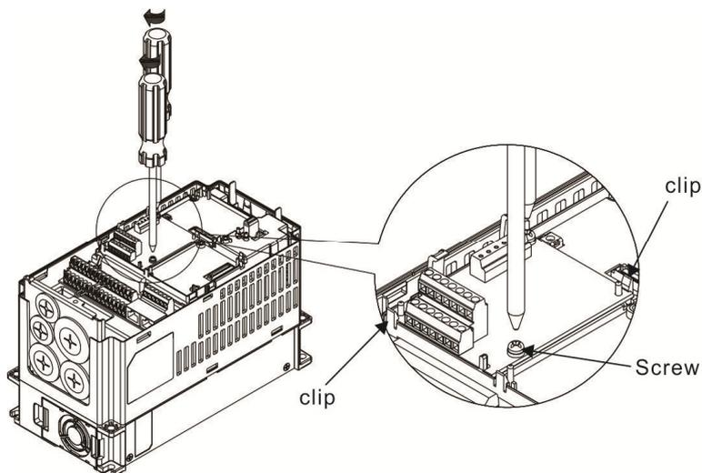
As shown in the figure on the left. Fasten, the screw after the PCB is clipped with the holes.
