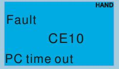
Fault<br>CE10<br>PC time out       | Modbus transmission time-out                                                                                                                                                                                                                                                  |                                                                                                                                                                                         |
