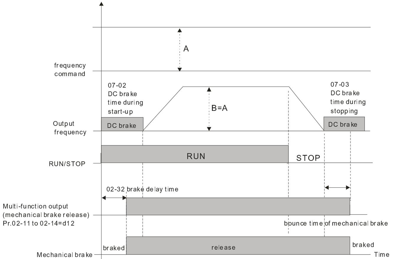
If this parameter is used without DC brake, it will be invalid. Refer to the following operation timing.
