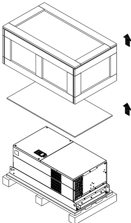
Remove the crate cover, EPEs, rubber and manual.
