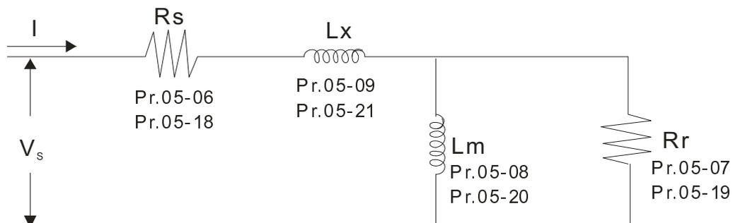
✳ If Pr.05-00 is set to 2 (static test), user needs to input the no-load current value of motor into Pr.05-05 for motor 1/Pr.05-17 for motor 2.
