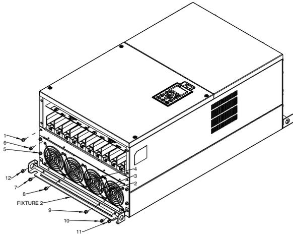
2. Loosen 12 screws and remove Fixture 2.
