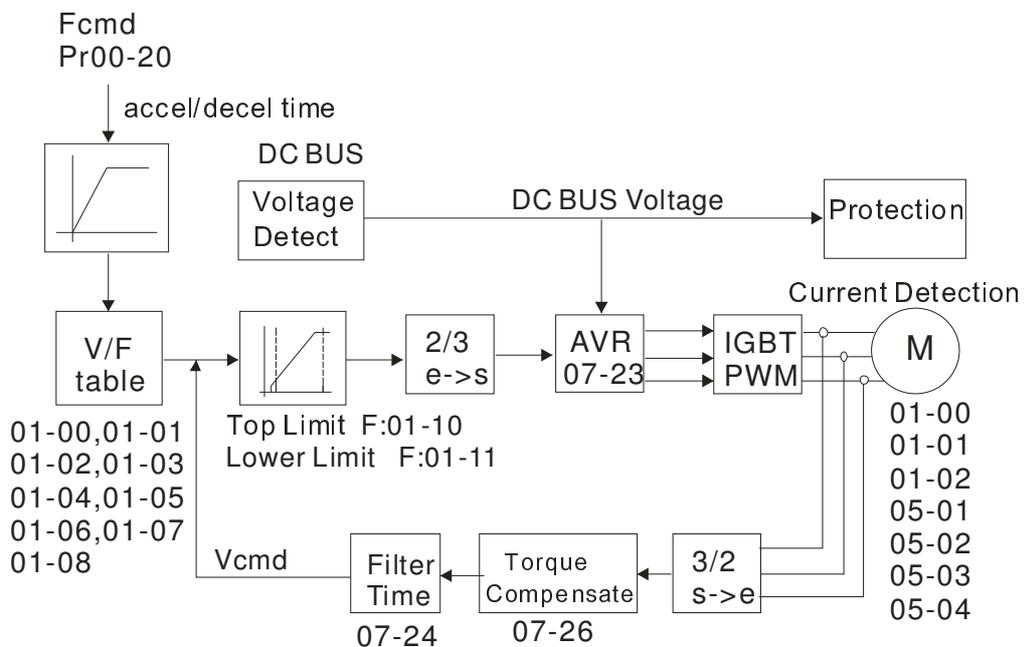
📖 When setting Pr.00-11 to 1, the V/F control + encoder diagram is shown as follows.
