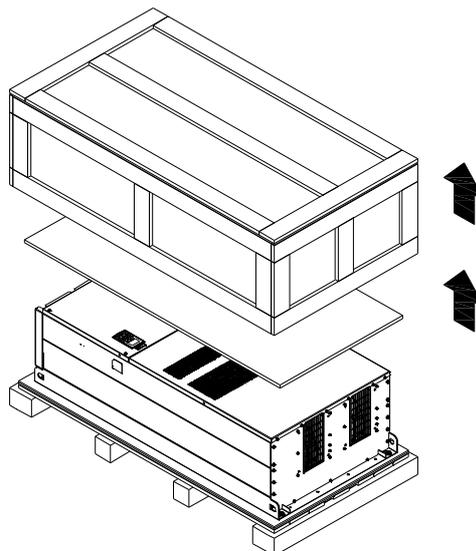
Loosen the 6 screws on the top then remove 6 metal washers and 6 plastic washers as shown in figure below.
