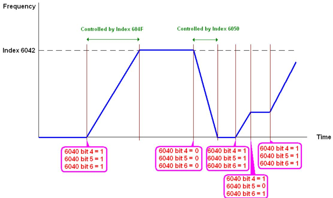
NOTE 01: To know the current rotation speed, read 6043. (unit: rpm)
