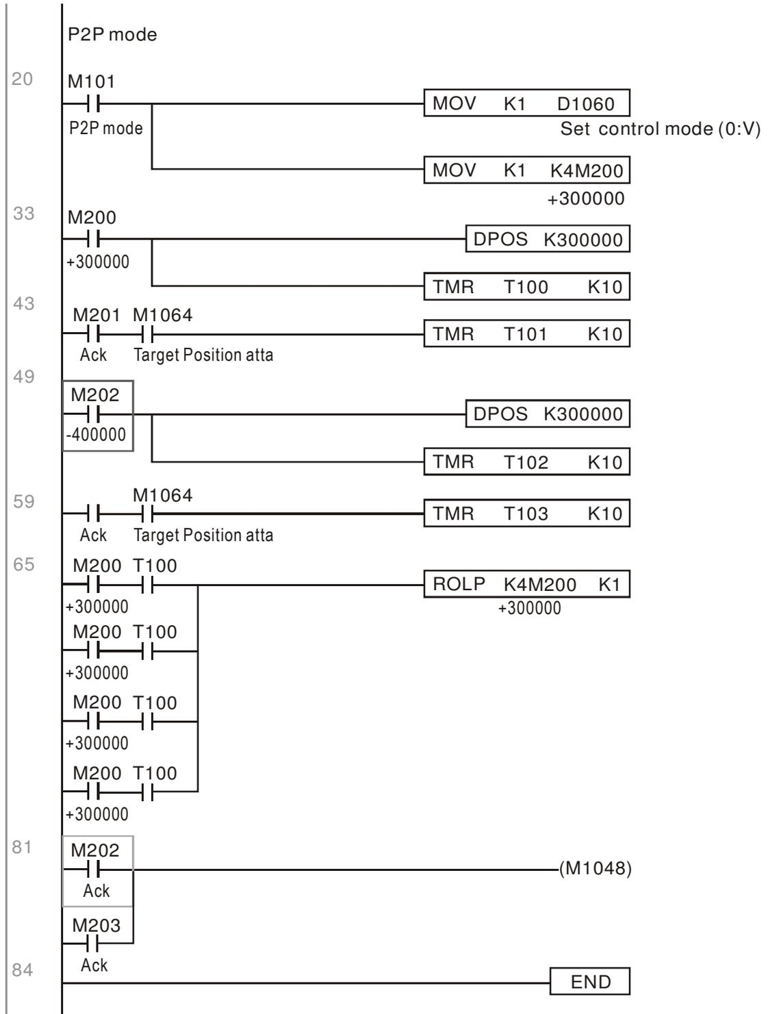
※ If homing is not needed in an application, the first and second parts can be skipped. However, the M1040 condition from Part 1 must be included, and the writing method in Part 1 involve the use of X2 to achieve direct access. In addition, when M101 is used at the beginning of Part 3 to set the control mode, it can be rewritten as M1002, which will put the PLC immediately into the position mode when it starts running.
