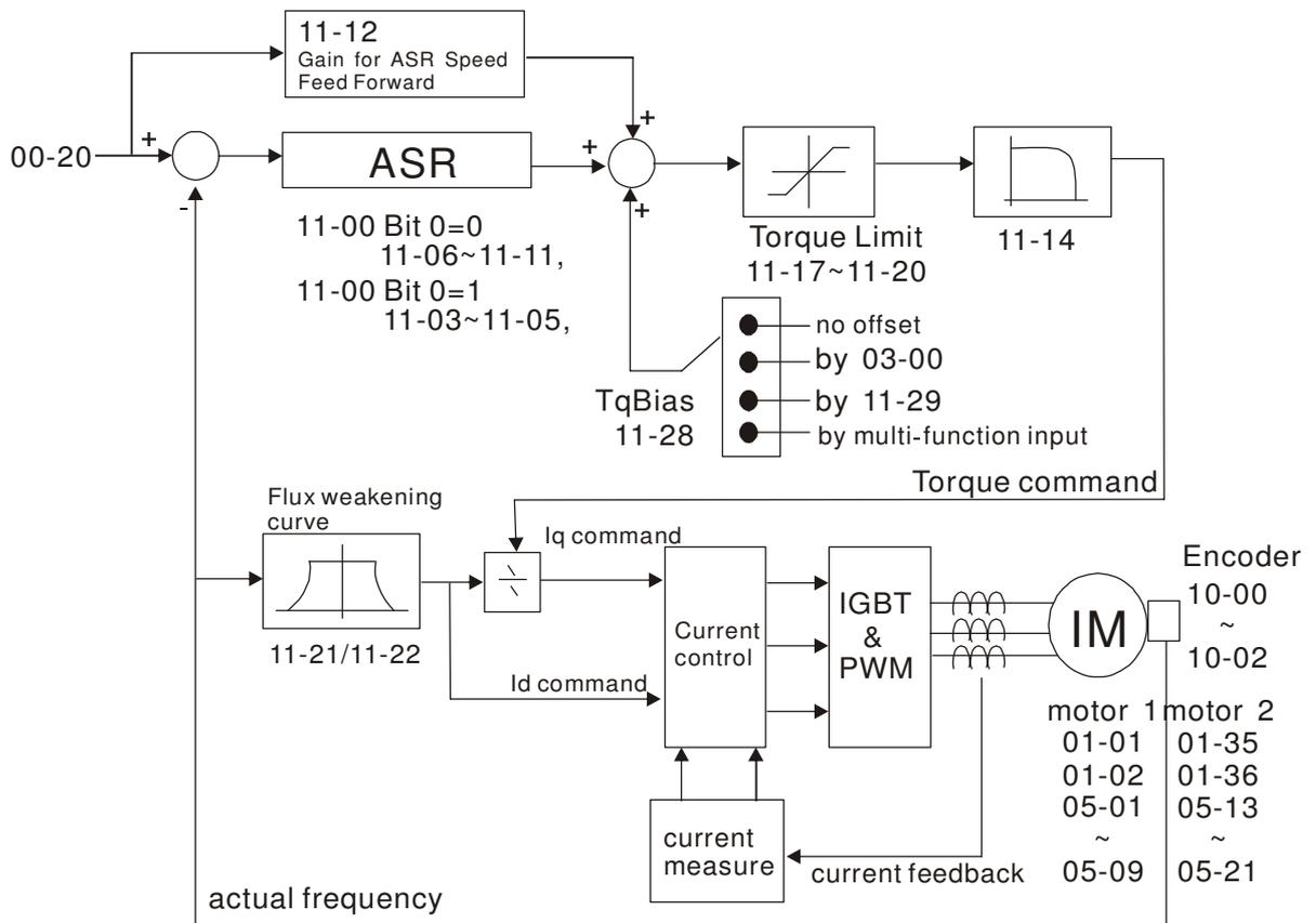
When setting Pr.00-11 to 4, the FOCPG control diagram is shown as follows.
