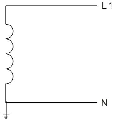
4 No stable neutral grounding in a three-phase autotransformer configuration
