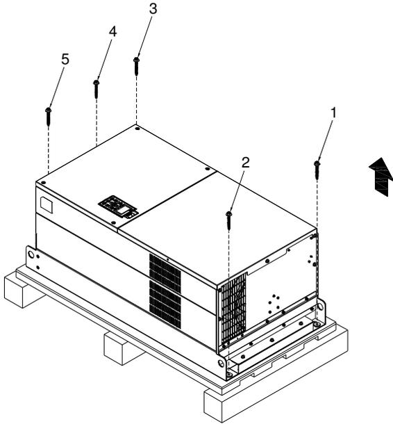
Loosen the 12 screws and remove the wooden plate.
