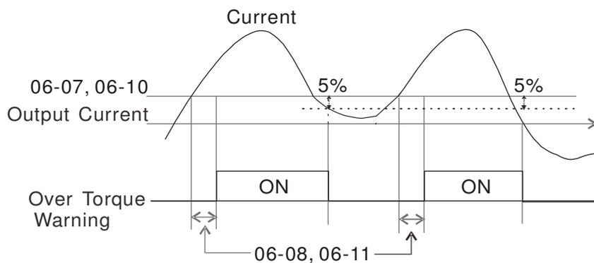
📖 NOTE03: When Pr06-06 or Pr06-09 is set to 2 or 4, the motor drive will have the ot1/ot2 fault after Over Torque Detection. Then the motor drive stop running until it is manually reset.
