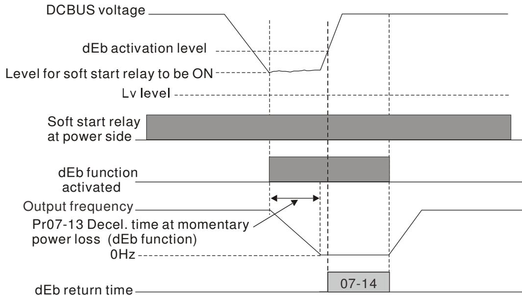
Note (1) When Pr07-14 is set to 0, the motor drive will stop and will not accelerate to the frequency before dEb even the power is on again. But when Pr07-14 is NOT set to 0, then a command of zero speed will be sent to wait for power on.
