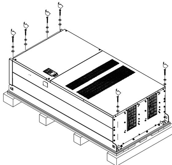
Lift the drive by hooking the lifting hole. It is now ready for installation.
