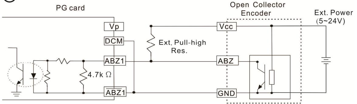
PG2 Wiring Diagram
